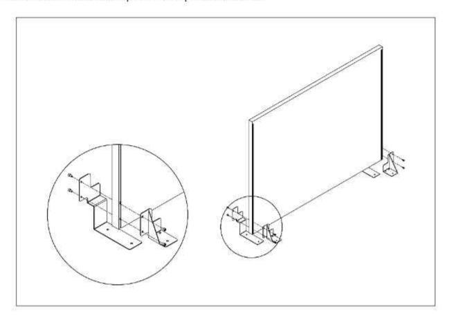
Step 3 - Fix the panel to the desk frame with 10 pcs M6x10 screws.
